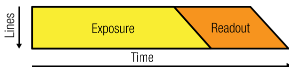
Figure 58: Global reset release mode - schematic
