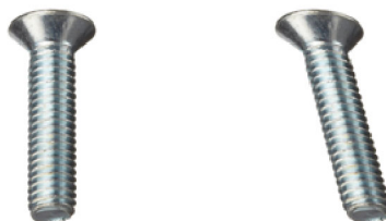
Figure 62: Rolling shutter mode image of a horizontally moved object
