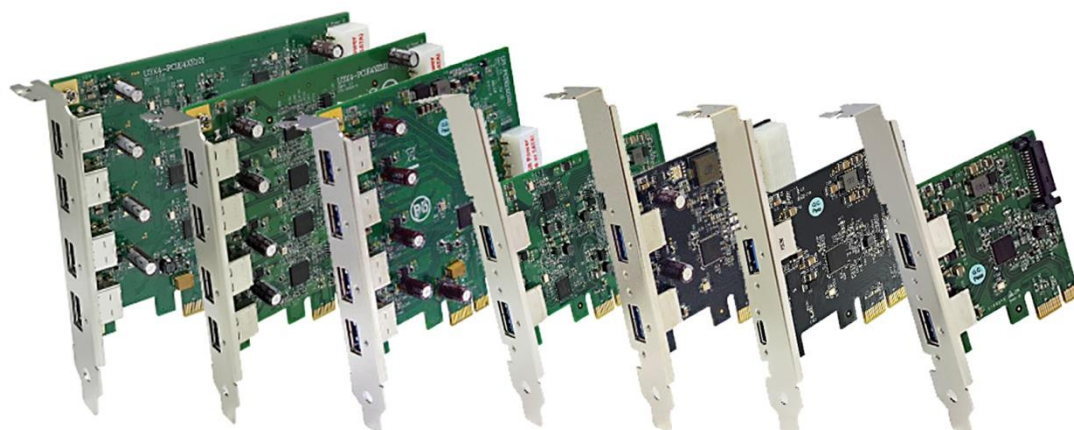
figure 3-40, USB3 host adapters
