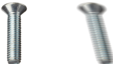
Figure 76: rolling shutter mode image of a horizontally moved object, long exposure time
