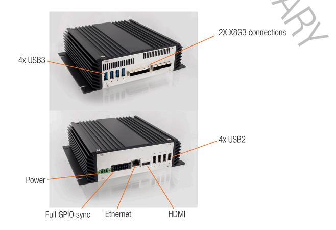
**COM express** computer by XIMEA allows development with the full range of cameras from USB to PCIe speeds in a compact platform. The switch contained inside allows many cameras input to the computer at full speed for processing, or saving. GPIO sync allows all cameras in the system to be trigered simultaneously.
