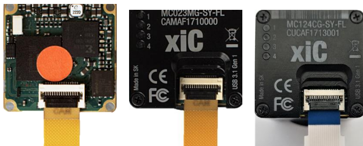
Figure 7-5, xiQ (left) and xiC (right) – camera side, correct FPC cabling
