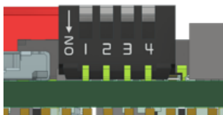
Figure 2-4, TX2CB-MAIN, TX2 GPIO Switch
