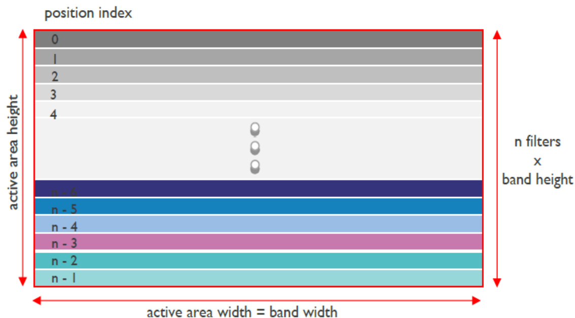
Figure 4-15, Principle structure of a line scan sensor (Source: imec)
