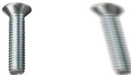
figure 4-6, rolling shutter mode, image of a horizontally moved object, long exposure time
